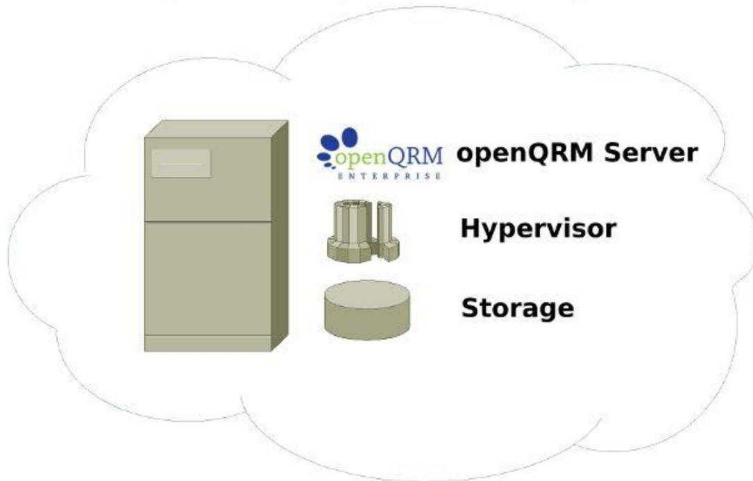
When using a “single-system openQRM setup” the storage-component, a Hypervisor and openQRM Server itself are installed on a single physical system. In this setup the openQRM system acts as the storage server and virtual machine provider. Therefore, here some special configuration recommendations and requirements especially for the single-system setup:
